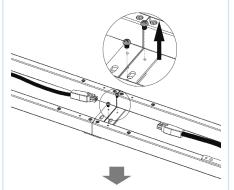
Attach the fixing plate to the frame using the two removed screws and tighten all screws with a proper screwdriver.
