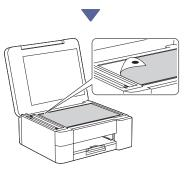
Place the Adjustment Sheet face down on the scanner glass, making sure the black circle is in the top left corner of the scanner glass, as shown.
